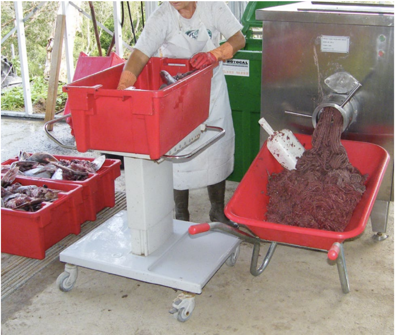
Figure 10. A small-scale tuna by-product processing facility, grinding tuna by-products into fertiliser (BioAgri-NC). Image from Bergè et al. , 2014, © Secretariat of the Pacific Community, 2014.
